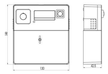
Fig. 4 – Meter fixing dimensions.
