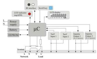
Fig. 1 - Meter block diagram
